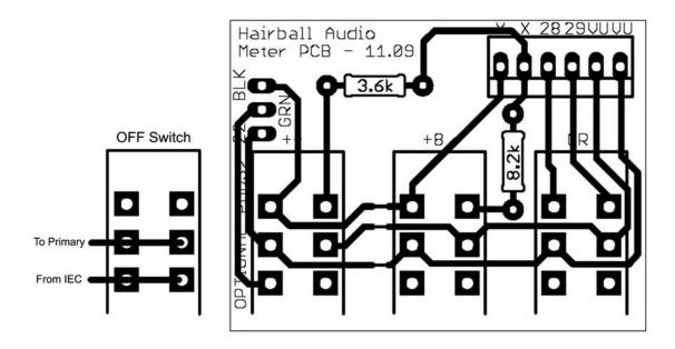
If using the on/off configuration, please be sure the switch specifications meet the requirements of the mains voltage in your region. You may choose to use the mains neutral for power switching to reduce excess voltage on the switch. Wiring in parallel will double the current handling capacity of your switch.
